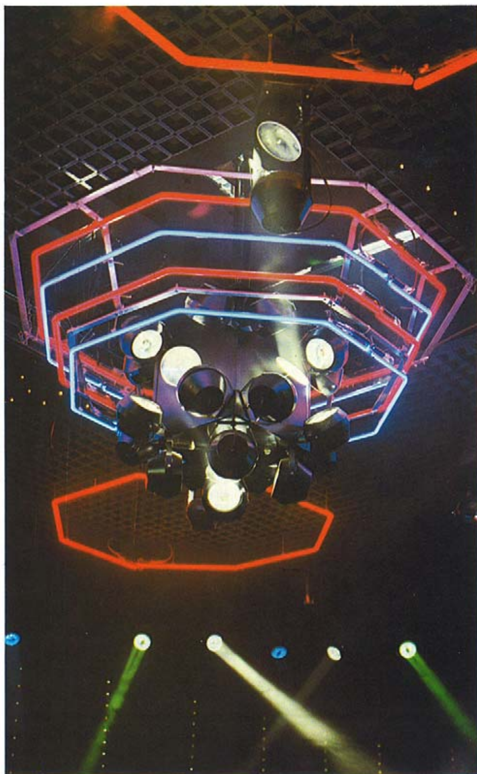
Supertrilus on a hydraulic ram at Benjy's Night Club in the Mile End Road, London.
